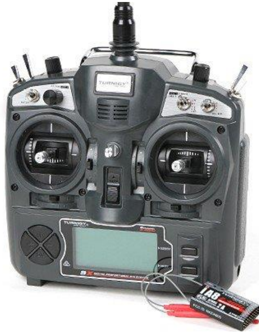
Figure 53: Turnigy 9X Transmitter with iA8 Receiver [109]
