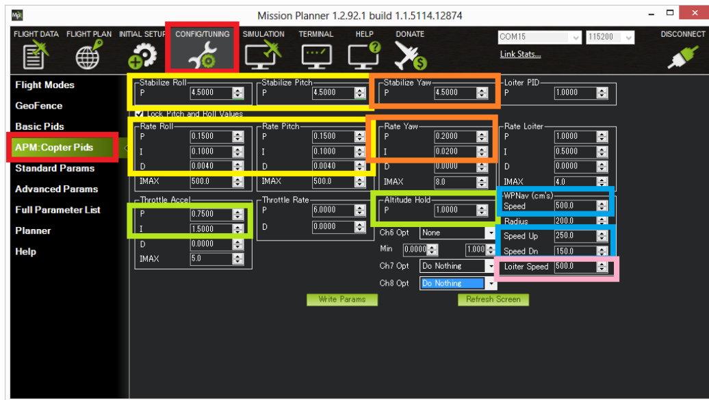
Figure 55: PID Tuning Page in Mission Planner [112]
