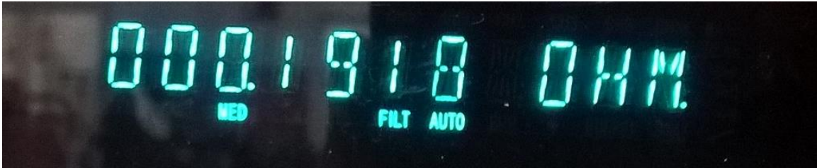
Figure 41: DJI Flamewheel PDB Resistance
